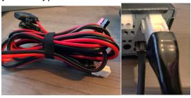
10. Connect the PowerPole end of the same red/black DC power cable to the [OUT] port of the PWRgate PG40S.
