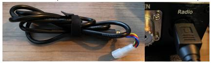
19. Connect the Molex connector end of the cable to the port on the main unit [TUNER].
